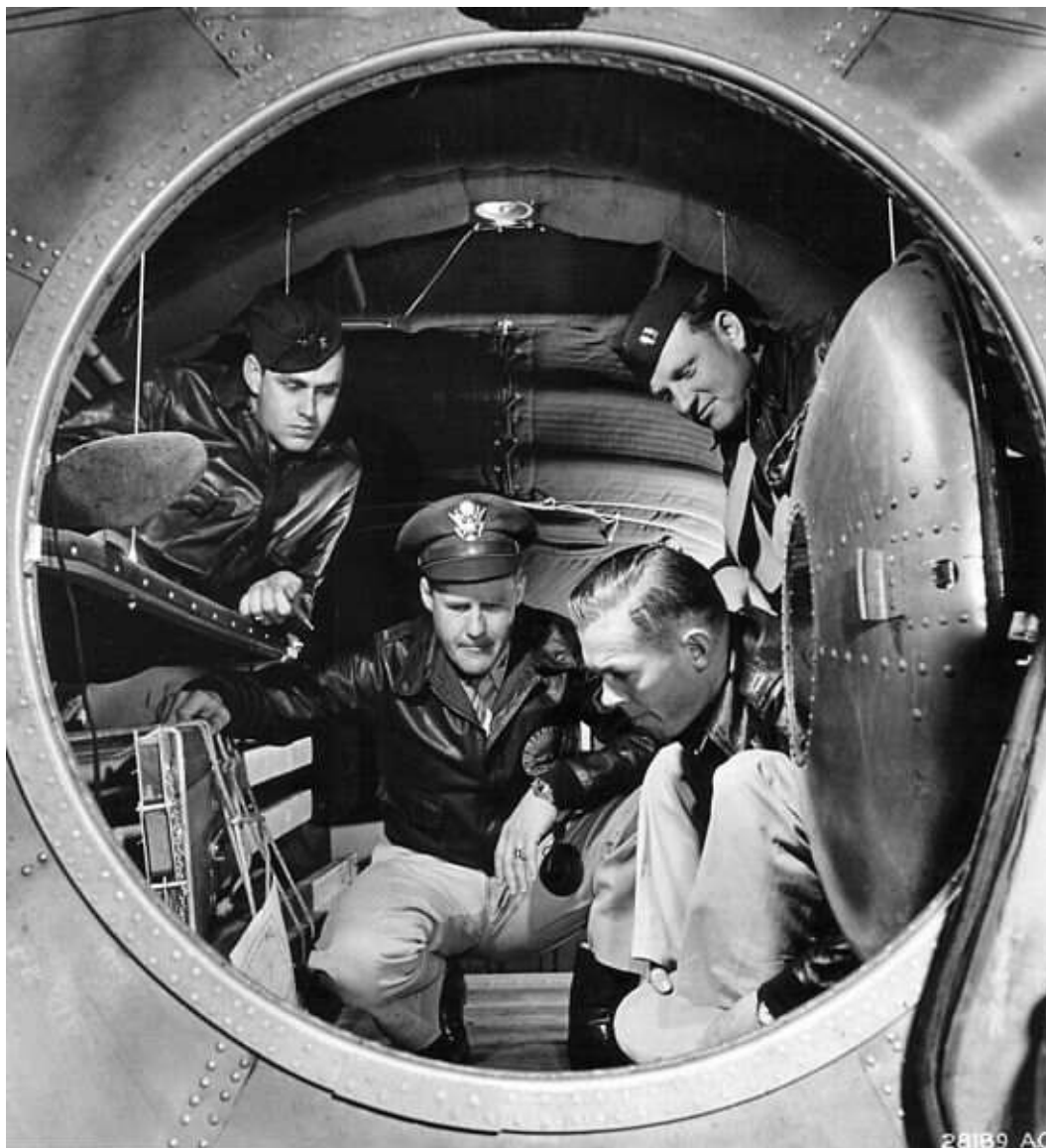
Figure 182: B-29 Super-fortress Rear Pressurized Hull (Crew Rest, 4 bunks)
