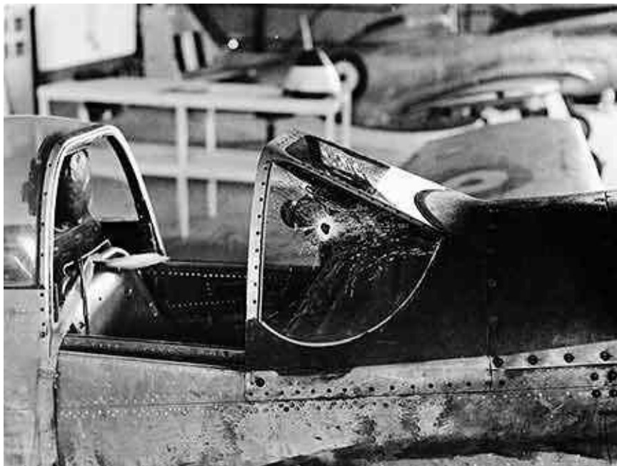
Figure 24: RAAF Mustang Flak Damage
