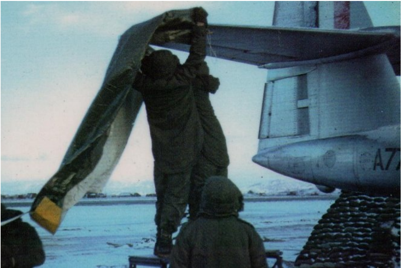
Figure 111: Groundcrew Sheathing Tailplane
