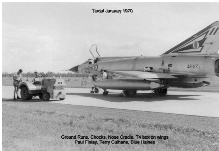
(A3-27 Ready For Ground Run. Note T4 test box on wing and cables to T4 probes. Personnel are Paul Finlay, Terry Culhane and Blue Haines, all Engine Fitters with 77 Sqn.)
