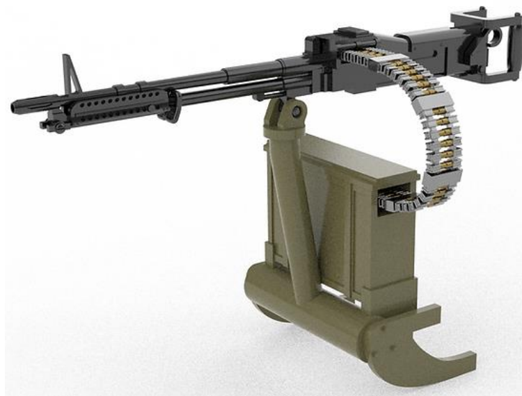
This drawing not to scale - note the short ammunition chute that was subject to twisting
