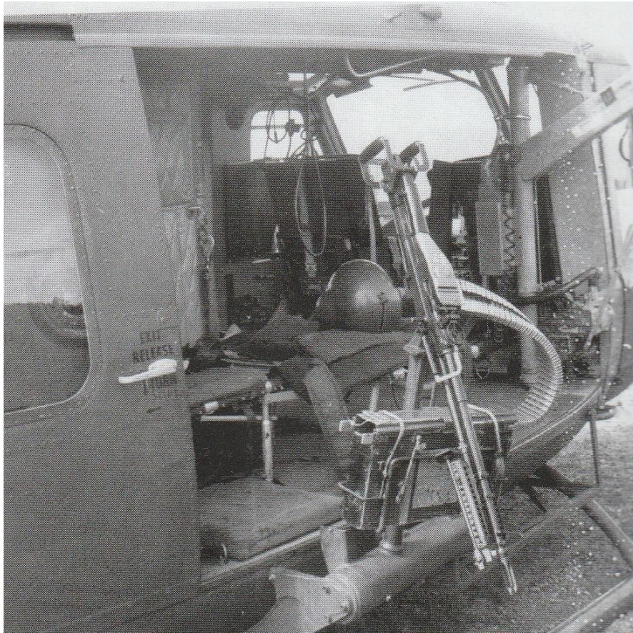
Note the straightened pintle post and rotating caged ammo bin
