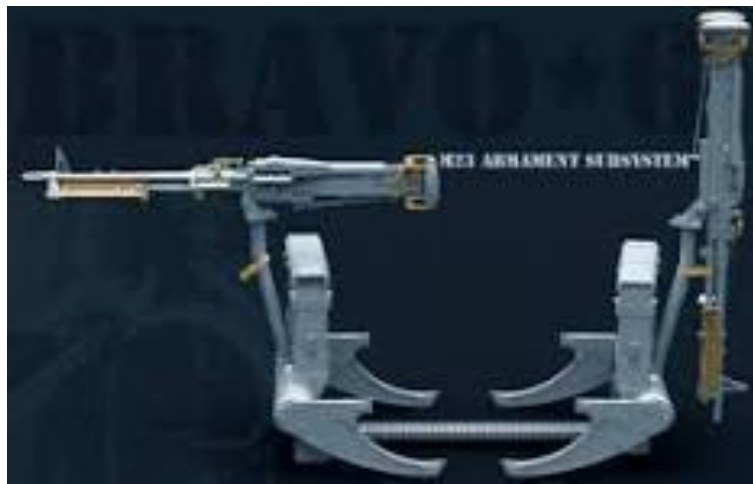
XM-23 Armament Sub-system - note the fixed ammunition bin and the bent pintle post
