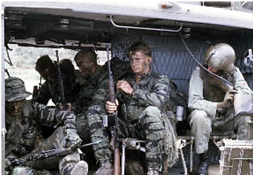
Note the rotating caged ammo bin and airflow deflector on the M-60D at far right of the image
